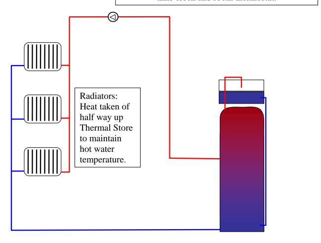
Linked or Hybrid system: Central Heating Circuit.
