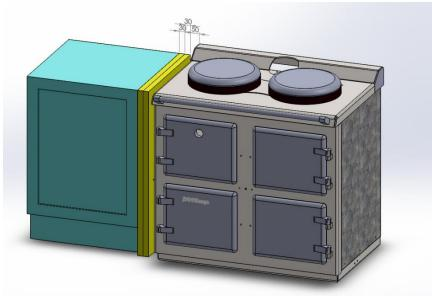
If you want to bring the cupboards closer, then you must ad insulation about 75mm thick. We recommend a material called calcium silicate boards which is very effective and we can supply 100cm by 90cm boards. These are 30mm thick.
