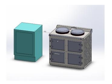
Minimum 450mm on left hand side of cooker to nearest cupboard or flammable material.
