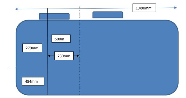
This diagram shows the position of the air inlet on the wood 5 oven cooker.
