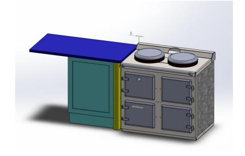
Note: It is because of this air gap that the 5 oven wood cooker is made with a left or a right hand firebox.
