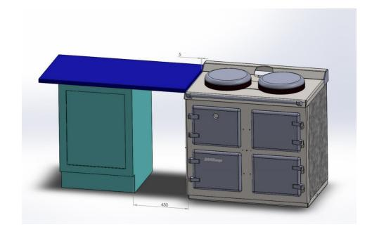
The work top can be taken up to the cooker still, but leave a minimum 5mm gap for expansion. If the work top is Formica, wood or other flammable material, you should leave the 450mm gap.
